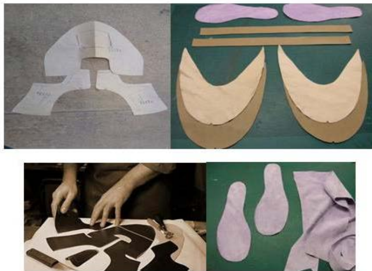
Figure 9: The Cutting Process of Uppers
